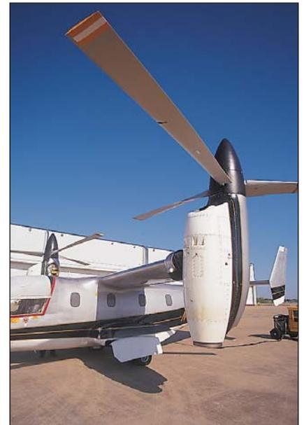
(Clockwise from top): The panel of the XV-15 proof-of-concept test platform features an EFIS display on the left for evaluation of differential-GPS steep approaches. The 609 will feature P&W PT6C-67A turboshaft engines, as opposed to the XV-15's Lycoming powerplants. Double-tire main gear will ensure smooth ground ops. The 609 will feature a T-tail, rather than the XV-15's lower horizontal tail surface, to eliminate aerodynamic buffet during transition.
