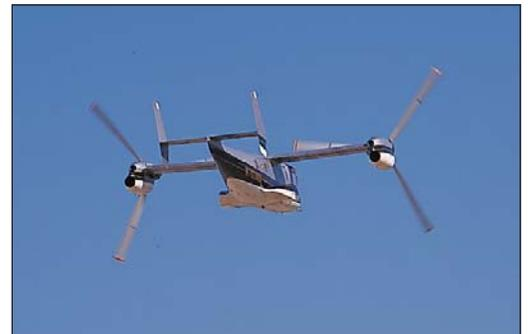
less than one min. Engine tilt control is managed with an easy-to-use “coolie hat” toggle switch on the collective. In “full forward,” the XV-15 feels just like an airplane.
