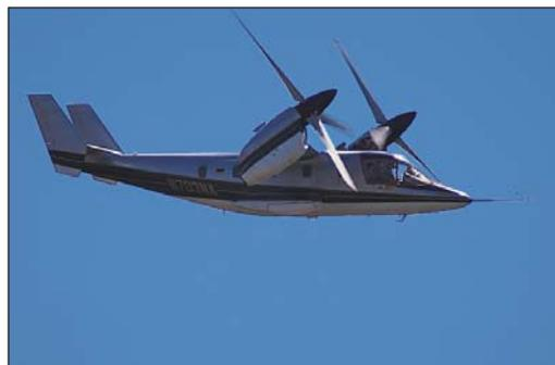
The conversion from a vertical nacelle angle to full-forward airplane mode can be accomplished in as little as 12-sec with a zero to 200-kt acceleration in
