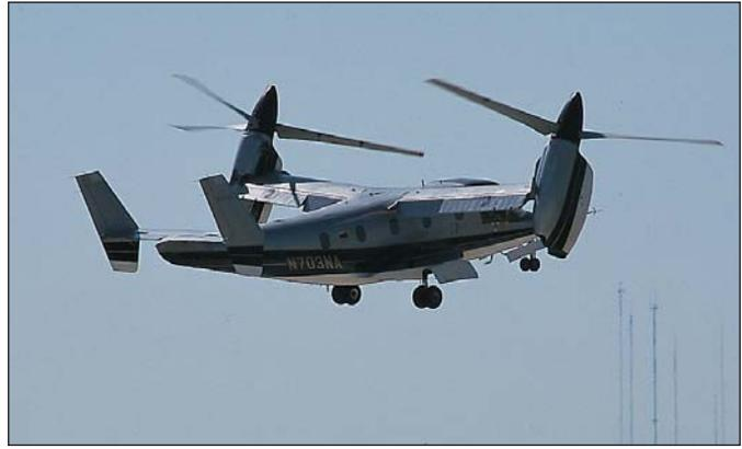
sions. The fuel burn required to hover, however, is more than in forward level flight at 240 kts. So to save fuel, and to operate quieter, you may want to do a running STOL takeoff at 60 to 75 nacelle angle when possible.
