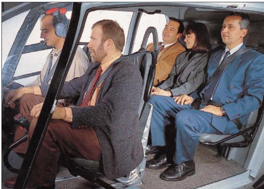
Visibility for both pilot and passengers is excellent within the EC120B's partitionless cabin (above). This new entry-level Eurocopter is well suited to police, utility, tourism, news-gathering and EMS applications. The EC120B's Turbomeca Arrius 2F turboshaft engine (left) develops 504 shp on takeoff and 449 shp of maximum continuous power.
