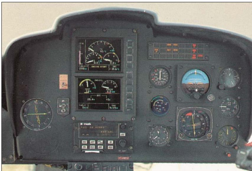
New flightdeck display technology on the EC120B centers around a fully-duplex vehicle and engine multifunction display (VEMD). First limit indications are clearly presented on takeoff and during normal flight operation to greatly reduce pilot workload.
