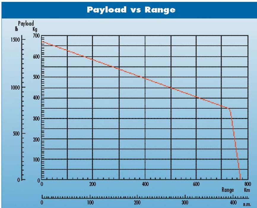
With a typical payload of three passengers, the EC120B can achieve a range of approximately 400 nm, which equates to about four hours of endurance.
