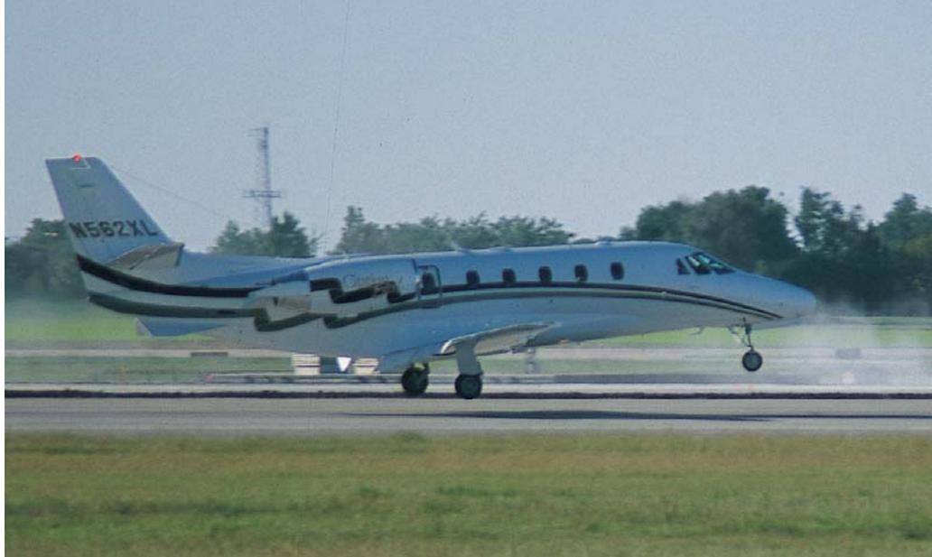
At the Excel's maximum landing weight and standard sea level conditions, the landing distance of the light jet is a short 3180 ft.
