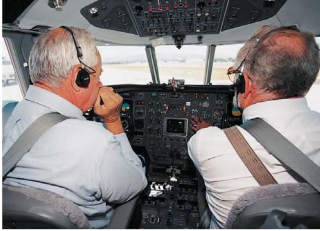
Lacy listens to Bow explain the 731 Falcon 20B's features, which include a direct vision window as well as a parking brake handle prominently positioned on the glareshield.
