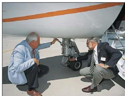
Lacy and Bow inspect the 731 Falcon 20B's nosewheel gear (L) during a preflight walkaround before checking out the aircraft's external baggage mod (R), which provides an additional 30 cu ft of storage capacity.
