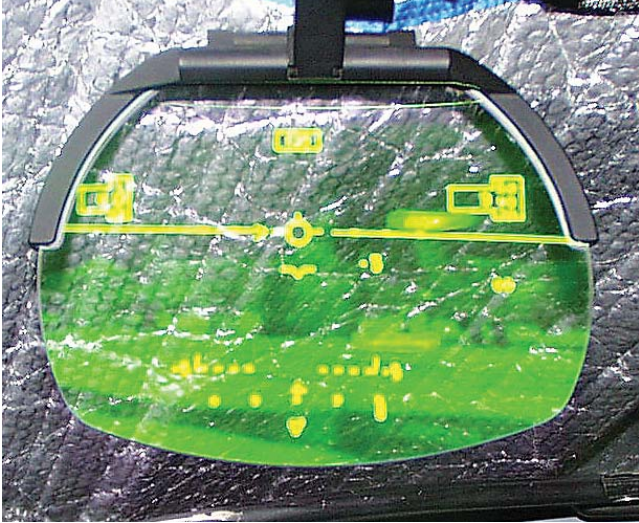
Here is a real time image transmitted from an IR camera mounted in the nose of a Gulfstream V to the HUD on the flightdeck. Gulfstream is offering the Kollsman EVS married to a Flight Dynamics head-up display system (HGS).
